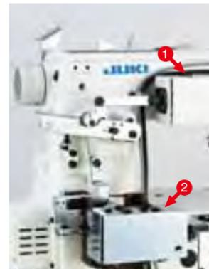
1 Presser lifter drive mechanism magnet
