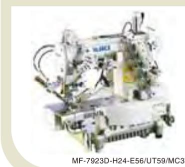
The machine is best-suited for the hemming of stretchy new material such as T-shirts, underwear and sportswear, etc. The machine produces seams with no semi-cylindrical swells by performing sewing while making the feeding lengths of the right and left needle threads equal. The sliding presser foot prevents the material hem from twisting during sewing and further eliminates oblique-feeding of the material in terms of its texture.
