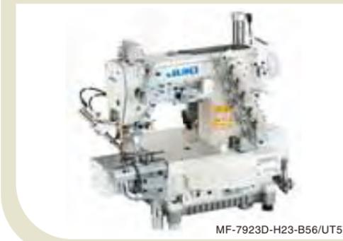
This model is best suited to hemming processes for sleeves and the bottoms of T-shirts, Polo shirts, etc. It comes with a left hand fabric trimmer for trimming fabric in parallel, at all times, to the seam with consistency. The upper knife stroke can be adjusted with ease.
