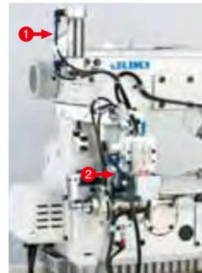
1 Presser lifter drive mechanism air cylinder
