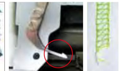
New cloth guide / The new cloth guide helps the machine perform hemming while keeping the hem width consistent.
