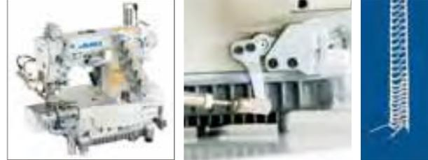
The needle thread tightening mechanism helps produce well-tensed seams even when the machine performs short stitching.
