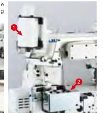
1 Presser lifter drive mechanism magnet
